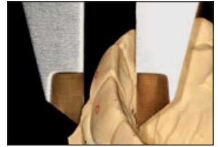
Fig 11 The facial-palatal width was measured using a digital caliper sensitive to 0.01 mm at each measurement point.
